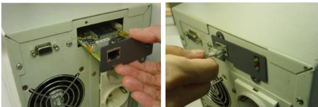
Fig.6. Internal NetAgent Installation
