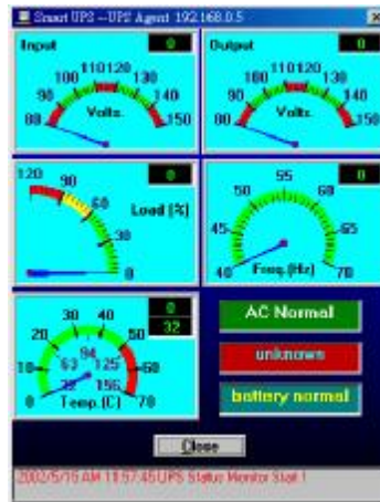
Fig.36. SNMPView: RS232 UPS status
